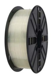
Material: PLA, 1.75 mm diameter Weight: 1 kg/spool (2.2 lbs) Length: approx. 330 m Density at 21.5°C: 1.25 g/cm3 Melt Flow Index at 10min, 2.16 kg: 5
